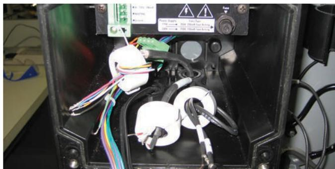
Figure 11: Ferrite Installation
